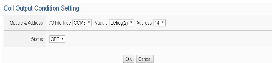
Figure 10-14 : Coil Output condition setting page
